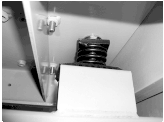
Figure 35: FanMatrix™ Shipping Bolt
